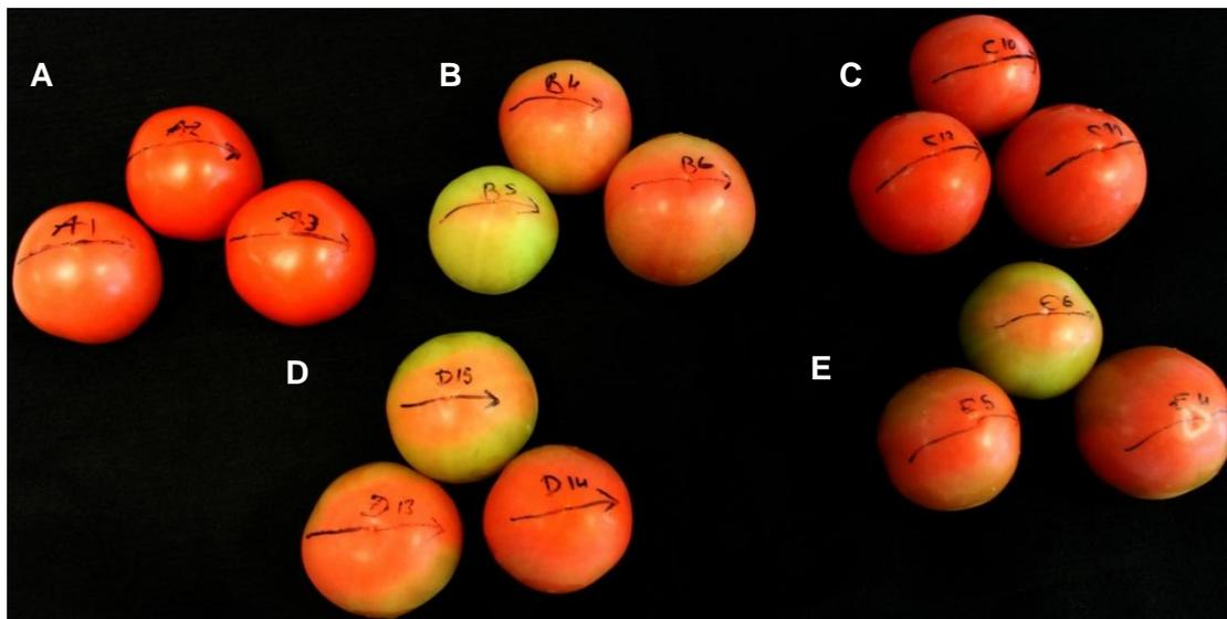
**Figure 2.** A representative sample from the fruits treated post-harvest showing: **A)** Control fruit. **B)** Conventional treatment with the low pressure mercury source. **C)** An 8 pulse treatment. **D)** A 16 pulse treatment and **E)** A 24 pulse treatment. Black lines on the fruit run parallel to the direction of UV source exposure which highlights the dependency of full surface exposure for delayed ripening. (Scott *et al.*, 2016)
